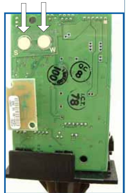
Front Face Of Board With Water (W) And Syrup (S) Only Buttons
