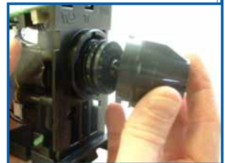
O-ring, Diffuser and Nozzle Replacement Replacement
